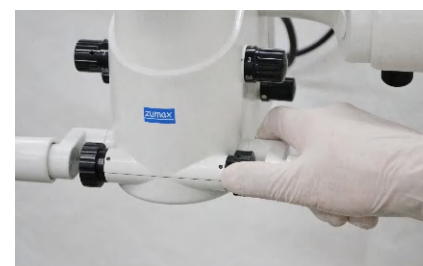
Adjust the fine focus knob
